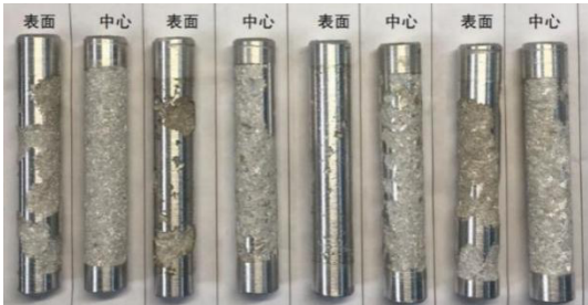
Nonuniform electrochemical dissolution morphologies
